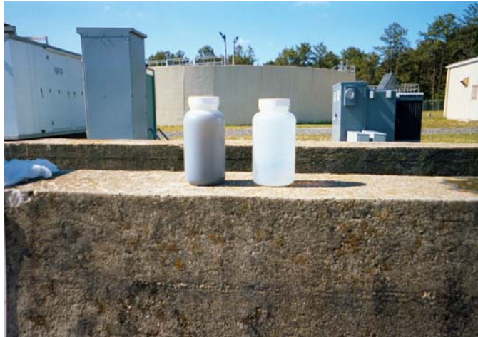
Influent & Effluent Samples at Brookhaven National Lab, Upton NY
